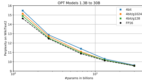
Figure 4: GPTQ at 4-bit with different group-sizes on medium sized OPT models.
