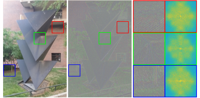
Figure 9. Visualization of camera trace in a single image captured by GalaxyN3. From left to right: original image, camera trace extracted by SiamTE, and patches in spatial and frequency domains.
